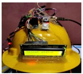
Fig. 3 .LCD displays helmet status.
