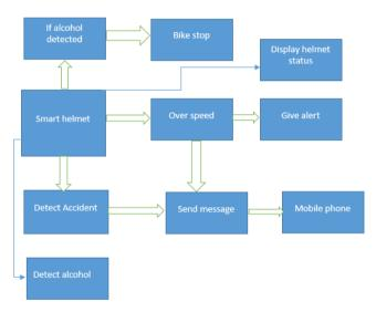
Fig. 1. Block diagram of Smart helmet
